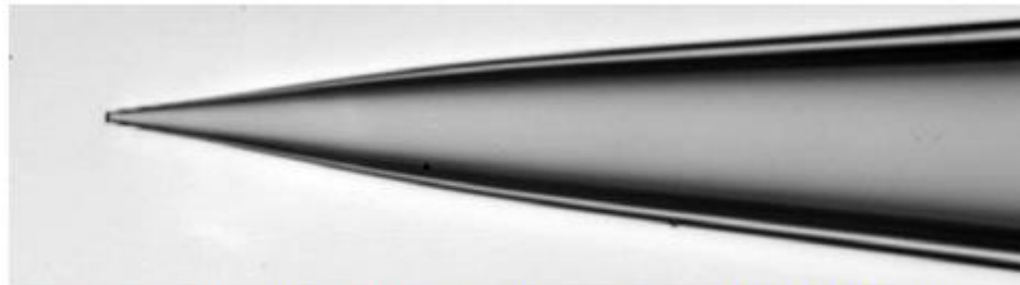
1.5mm x 0.86mm thick walled glass, ~2 \mu m Tip, 3-4mm taper (400X mag)
