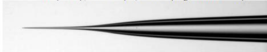
Image A (40x mag.) 1.0 x 0.5 thick walled glass (BF100-50-10) ~0.5 \mu m Tip, 4-5mm taper, one line program with 3 loops
